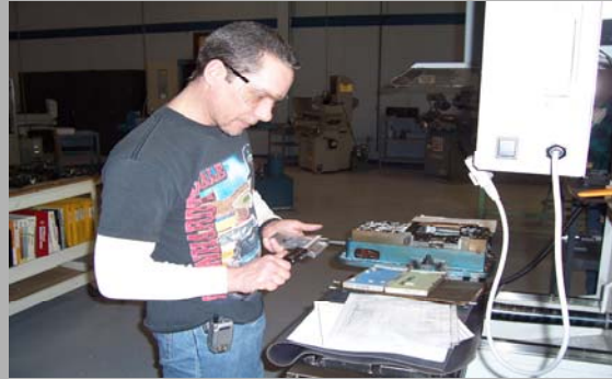
Russ uses calipers to check the size of a machined part and compares to the measurements indicated on the print
